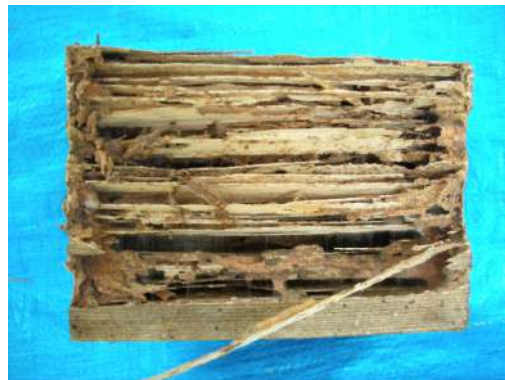
Damage example of non-treated western hemlock
