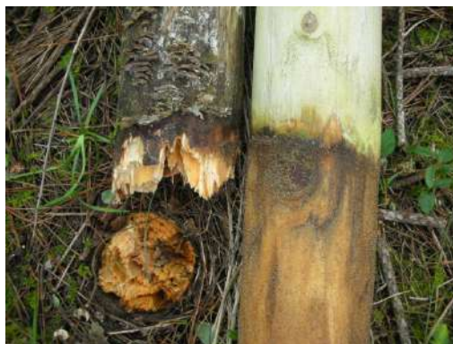
Magnified photo of the broken portion on posts Left: Non-treated wood (broken) Right: Marvel Wood
