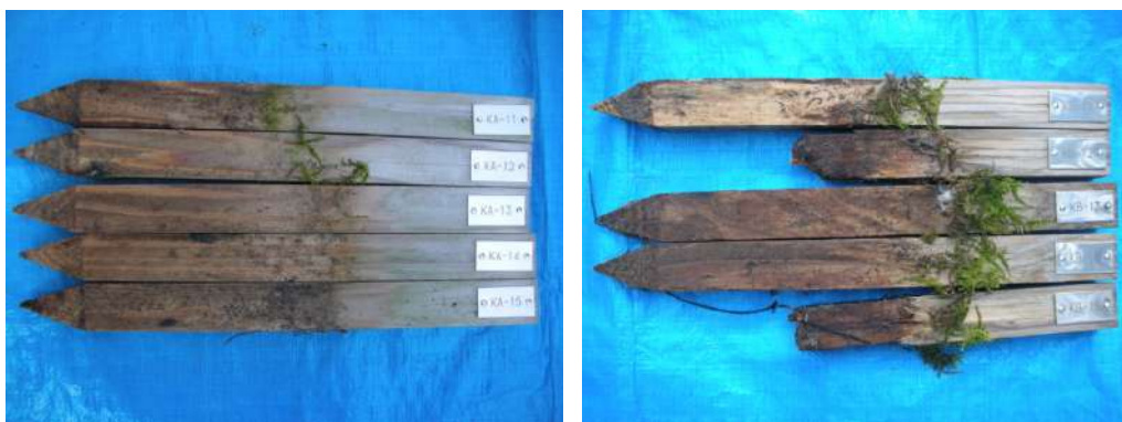
The test stakes after the test. (Left: Marvel Wood, Right: Non-treated wood)
