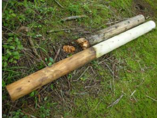
A look of the posts as of 2 years from the test start Top: Non-treated wood (broken) Bottom: Marvel Wood
