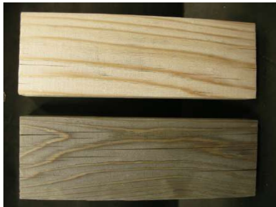
Results of the outdoor weathering test in one year
